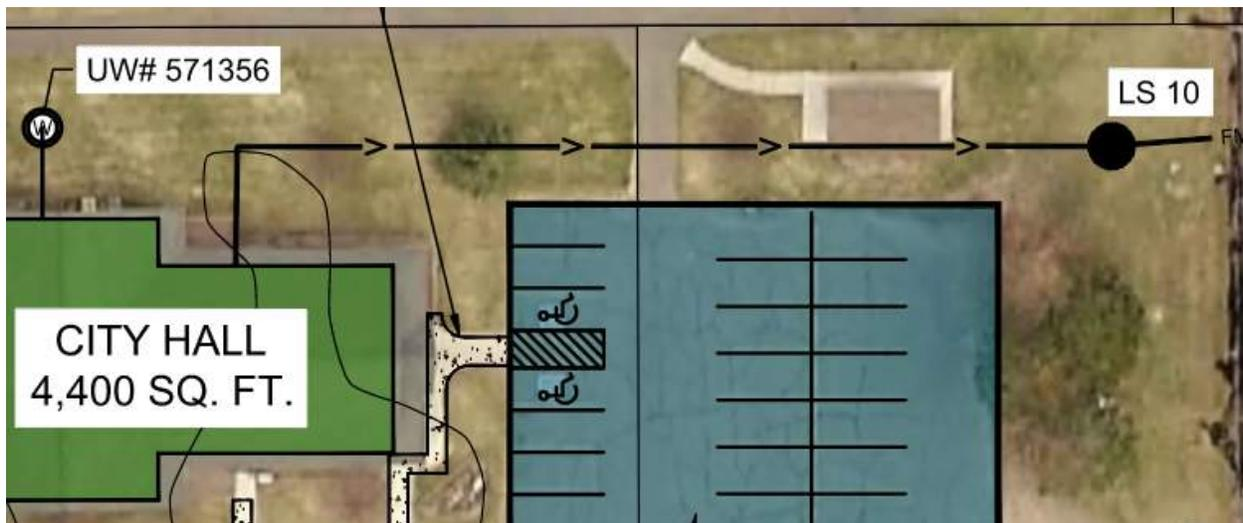
Photos: Approximate sanitary sewer service line and lift station location.
